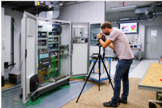
WKC - Test laboratory - Heat measurement
