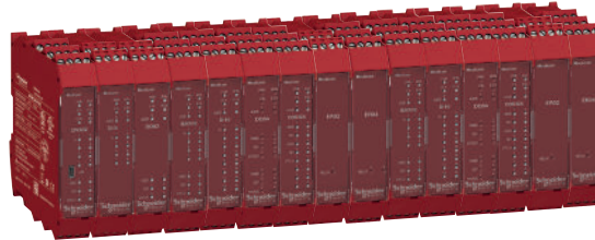
Maximum size of hardware: one safety controller CPU connected to fourteen expansion modules (1) via the backplane expansion connectors: 128 inputs + 16 OSSD pairs or 32 single channel OSSD + status outputs
