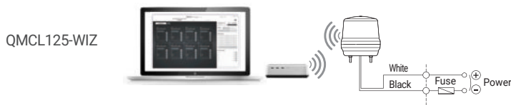
Ethernet connection via Gateway
