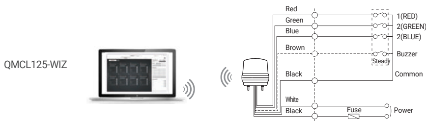
· Wiring Configuration for Signal Color
