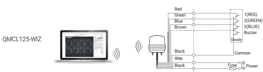
· Wiring Configuration for Signal Color
