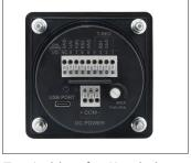
Terminal box for Signal phone panel(back side)
