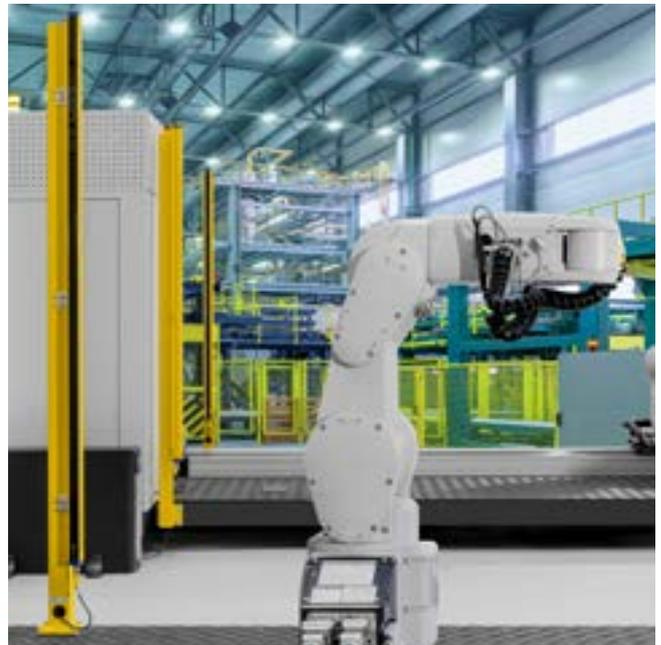
Safety devices are mandatory for operator protection in potentially hazardous areas, plants or machinery. Datasensing safety light curtains are used for the detection of finger, hand, arm, body, or presence detection in fixed applications; whereas safety laser scanners are recommended for area protection in static or dynamic applications, such as robotic cells and automated guided vehicles (AGV).
