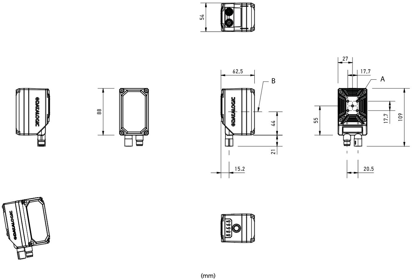
**P2X-SERIES MICRO LENS, ILLUMINATOR 14 LED (90° connection)**
