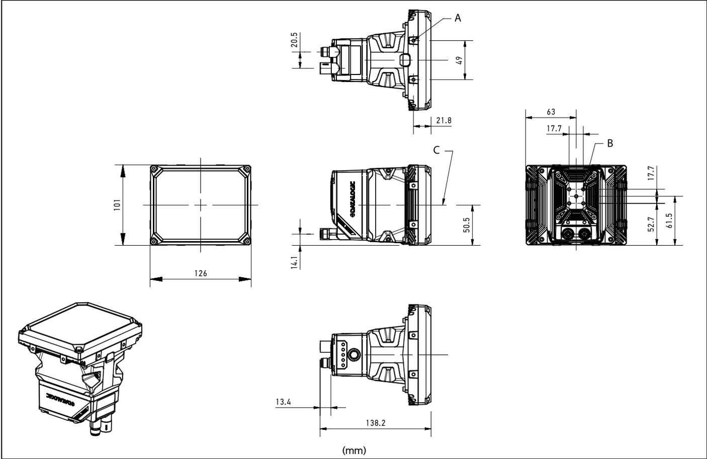
**P3X-SERIES MICRO LENS, ILLUMINATOR 14 LED or no illuminator (0° connection)**
