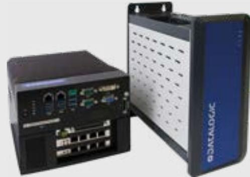
Rugged Industrial Machine Vision Processors providing the highest performance in image processing with unmatched flexibility through Ethernet (GigE Vision) connectivity and multi-camera support.
