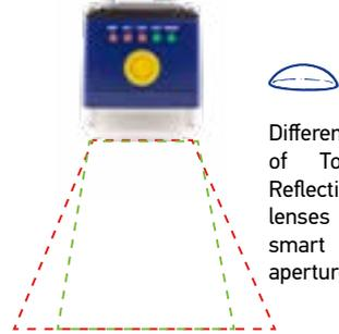
Different options of Total Internal Reflection (TIR) Led lenses to match smart camera lens aperture
