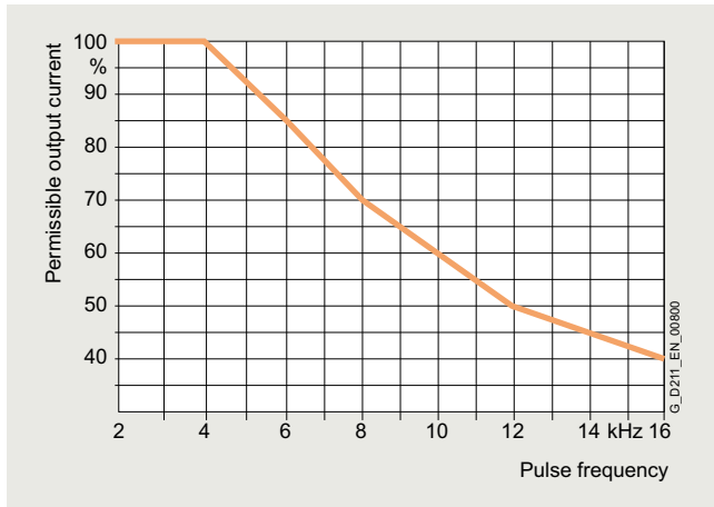
Permissible output current as a function of the pulse frequency, SINAMICS G220, at low overload (LO)
