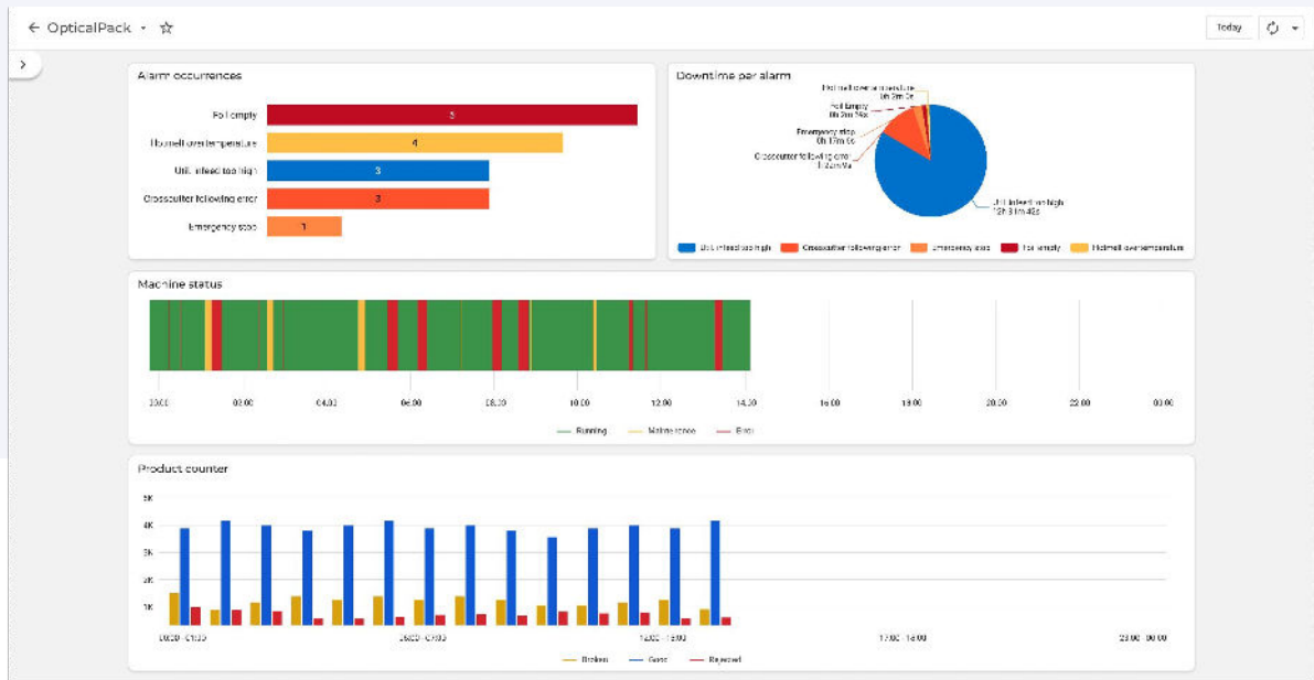
Analysis of downtime with machine status, alarm occurrences, and downtime per alarm.
