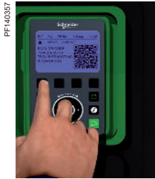
PF140357 Embedded dynamic QR codes generated on error detection
