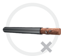
Remains of the conductor insulation on the stripped conductor
