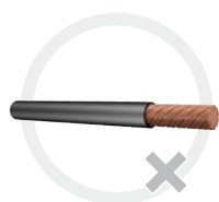
Excessively twisted individual wires
