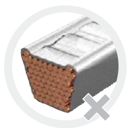
Formation of cracks at the sides. Sides split open
