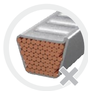
Asymmetrical crimping shape Burr formation on one side
