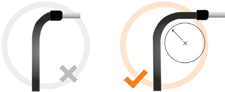
Risk of breakage due to overload
