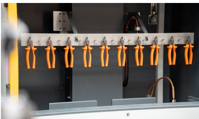
10,000 V test for 1,000 V safety for our cutting tools.
