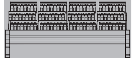
Field terminals view for ADV161 (Channels 33 to 64)
