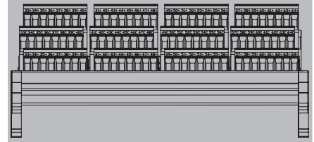
Field terminals view for ADV161 (Channels 33 to 64)
