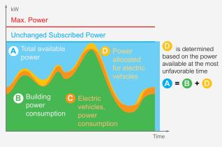
Setpoint "D" is fixed. The power is distributed between all connected vehicles.
