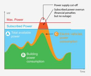
The installation of charging stations in an existing electrical installation can have a significant impact due to the power level required by electric vehicles to charge.
