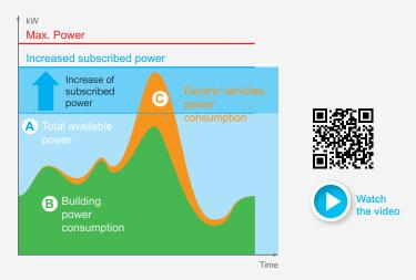
This solution consists of increasing the power subscribed to the energy supplier to maintain the same consumption model. It implies an increase in the cost of the subscription and the trigger threshold can be exceeded. Thus the continuity of service of the building could be impacted.
