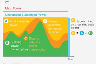
Setpoint "D" is adjusted in real time according to the consumption of the rest of loads in the building, to maximize the power allocated to charging electric vehicles.
