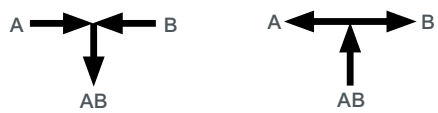
VB-8303 2½"...6" 3-Way Mixing Stem Up VB-8303 2½"...6" 3-Way Diverting Stem Up Flow is B Port to Common Bottom AB Port Flow is Common Bottom AB Port to B Port
