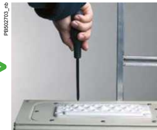
Make a Small Hole in the Membrane
