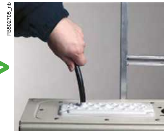
Pull the Cable or Tube Back Some 20 mm to Lock It
