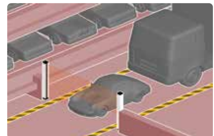
Detection of overall dimensional limits of vehicles for vehicle handling in automatic parking garages
