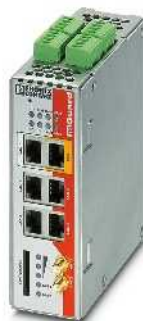
With firewall and VPN, managed 4-port switch, DMZ port, and 2nd WAN interface (US version)
