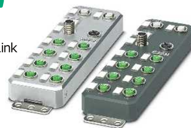
8 IO-Link ports, 4 digital inputs
