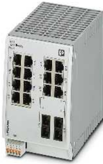
14 RJ45 ports and 2 fiber optic ports (multimode)
