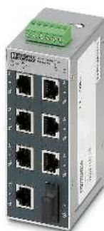
7 / 6 RJ45 ports and 1 / 2 fiber optic ports (multimode)
