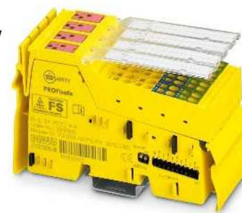
Digital output module, +/- switching
