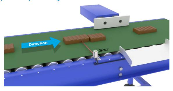
This function is designed to monitor that the length of an objects and the gap between the following object on a conveyor belt are within certain limits.
