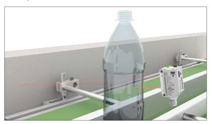
The 1 mm, visible, round, red laser spot is aimed at the background surface and taught in Dual Detection mode. The reflected distance and light intensity of the background is saved in the sensor as a reference. A change in the position or intensity of the reflected light caused by the presence of a bottle, will be detected by the sensor as an object (bottle).
