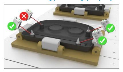
The small 1 mm visible round red laser spots are aligned on the background surface with the clips missing and taught in foreground suppression mode to recognize the background itself. If the clips are correctly mounted, they will prevent the sensor from seeing the background and thus the clips are detected.
