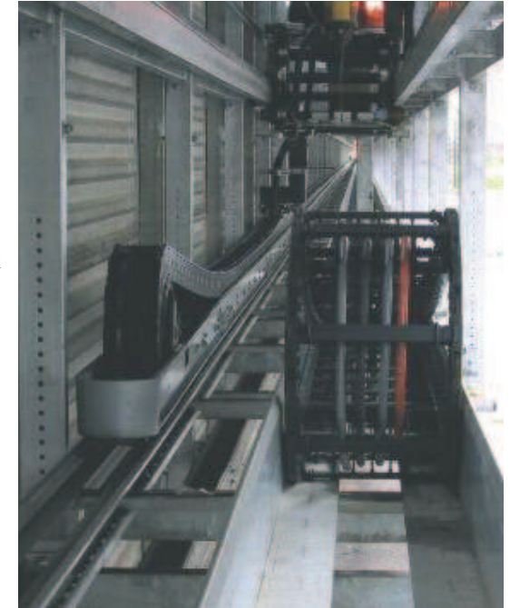
Chain testing rig for long travel: Tests at 8 m/s for 130 m travels.
