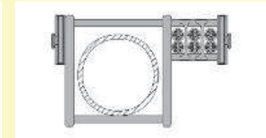
Larger split cross pieces. For the transportation of hoses of notable dimensions.
