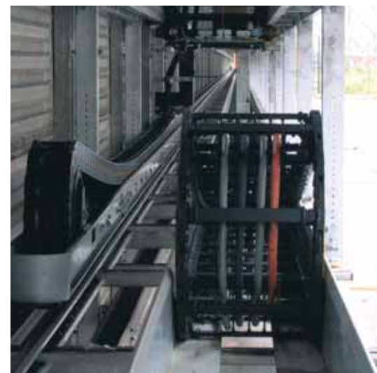
Chain/Cable testing rig for long travel: Tests at 8 m/s for 130 m travels.
