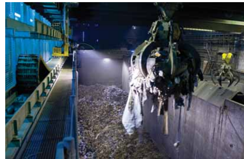
Nylon sliding chains type M80 installed on waste incineration plant "Vestforbrænding" in Denmark
